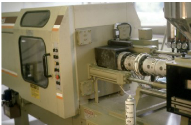
Fig. 2. A modern injection moulding machine with wear resistant barrel insert for ceramic injection moulding; the principle is similar to that used in metal die casting; injection moulding is a casting process.
